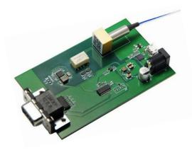
Agiltron offers Fiber Optic MEMS Tunable Filters with central wavelengths of 1060nm, 1310nm, 1550nm, and 2000nm. It is tunable continuously over a spectral range of up to 80nm at a speed of about 80ms. The wavelength tuning is actuated by driving a rotating MEMS mirror that is optically coupled with a grating and a dual fiber collimator. It is conveniently controlled with user-friendly GUI and control interfaces of USB or RS232.
